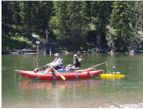
Figure 2. Cataraft, echo sounder, and acoustic Doppler current profiler used on the Snake River.
