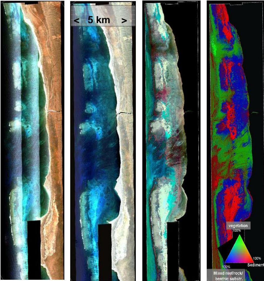
Figure 4: HyMap raw data (left) with atmospheric and sunglint effects. In the corrected image mosaic (right) no remaining artefacts are visible even at the boundary between two adjoining flight tracks.
