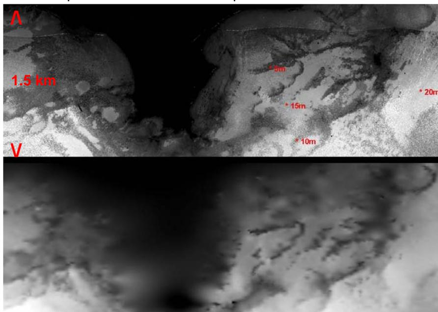
Figure 3: HyMap derived bathymetry subset (top) and comparison to gridded echo sounding derived map (bottom).
